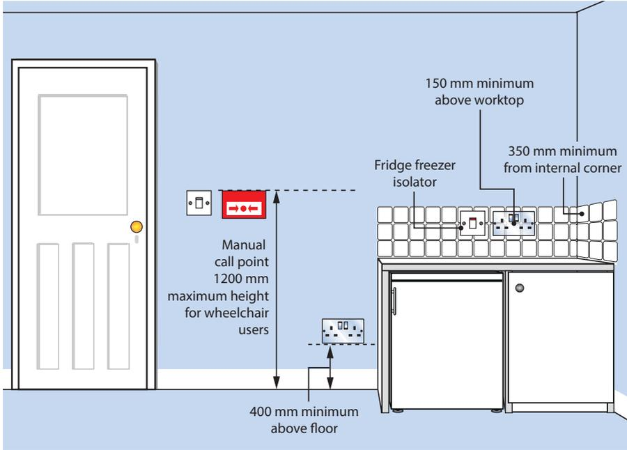
**Note:** Electrical accessories and controls should not be sited at more than 1.2 m above floor level (unless the need for a higher location can be demonstrated).
