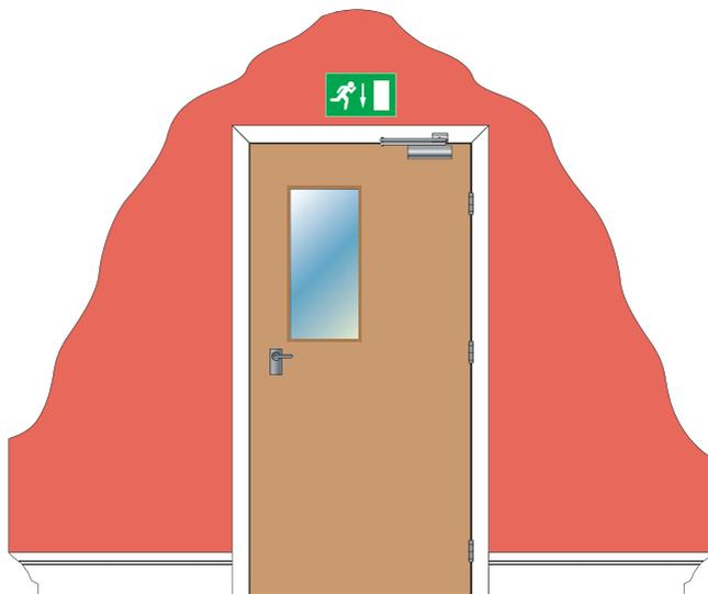
A self-closing fire door may be fitted with an electrically operated hold-open device, as specified in *BS 5839-3: Fire detection and alarm systems for buildings. Specification for automatic release mechanisms for certain fire protection equipment*. However, where an electrically operated hold-open device is installed, it should de-activate on operation of the fire alarm.
