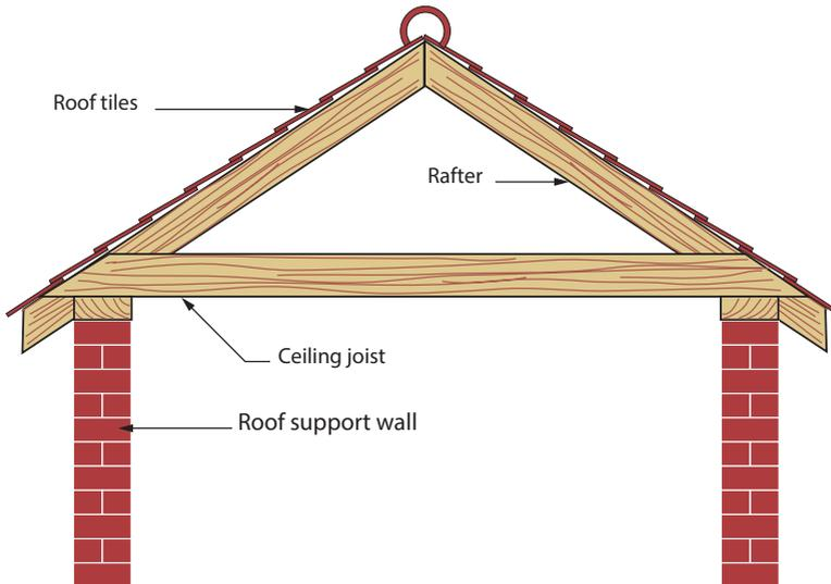
Note: Notches or holes should NOT be cut in roof rafters
