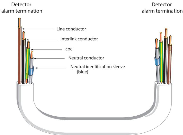
**Note:** Cables that are used to supply and interconnect the smoke alarm system in a typical dwelling (that is a dwelling with no floor area exceeding 200 m<sup>2</sup>) are not required to be fire-resistant.
