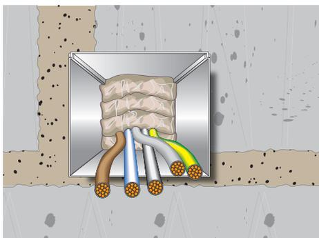
Internal sealing of wiring systems (Regulation 527.2.2)
