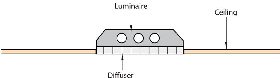
Where lighting diffusers form an integral part of a fire-resisting ceiling, which has been satisfactorily tested, the amount of thermoplastic material is unlimited.
