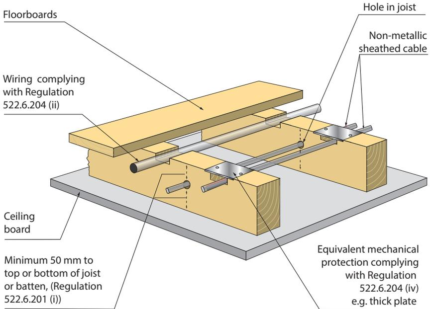
The position and size of holes and notches in joists etc is subject to the requirement of the Building Regulations
