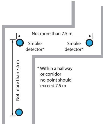
Detectors should be positioned so that they are accessible for maintenance and testing purposes, and should not be sited above staircases or in any other location that may be difficult or unsafe to access.
