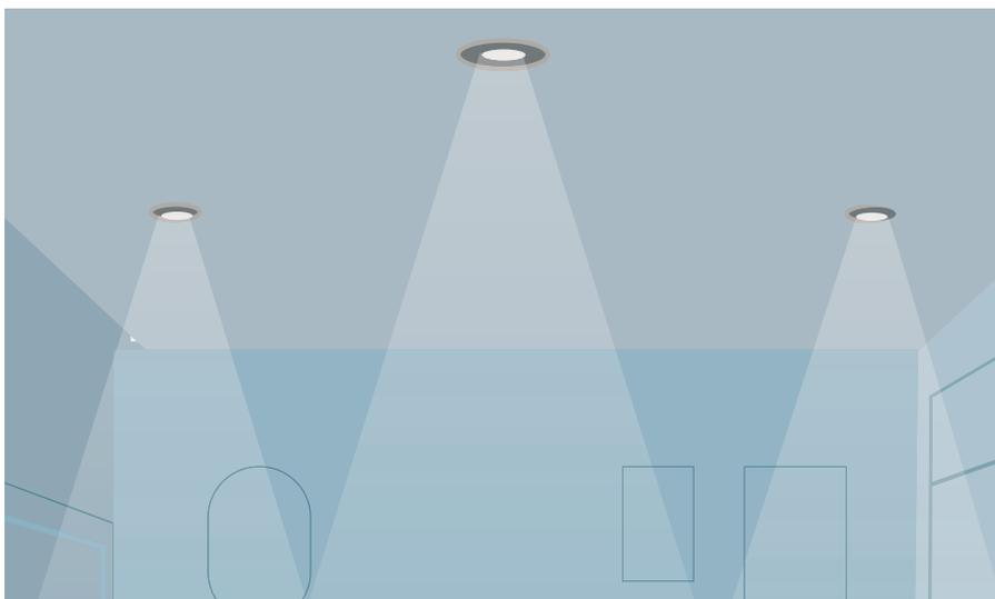
Downlighters installed at a greater density than one per 2 m<sup>2</sup> should be supported by test evidence undertaken in accordance with Annex B6 of *Example Constructions and Generic Internal Constructions*.
