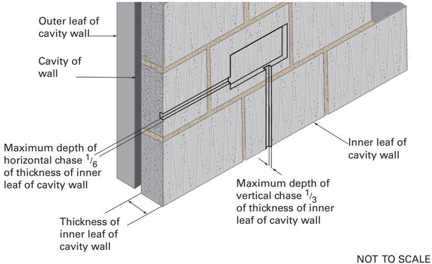
Vertical chases should not be deeper than  $\frac{1}{3}$  of the wall thickness or, in cavity walls,  $\frac{1}{3}$  of the thickness of the leaf, and horizontal chases should not be deeper than  $\frac{1}{6}$  of the thickness of the wall or leaf.
